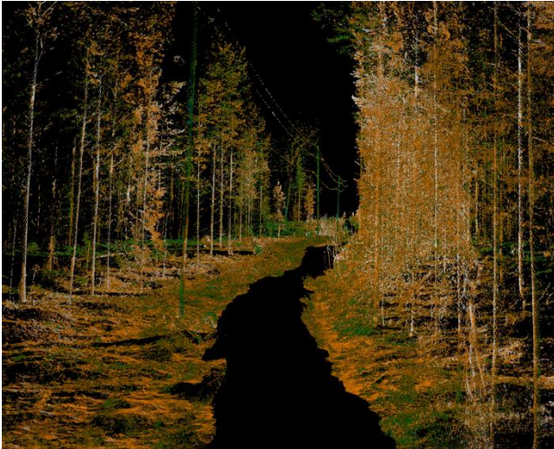
Figure 12. Example of a point cloud picture from a forest and an electric line (Pointcloud.fi)
